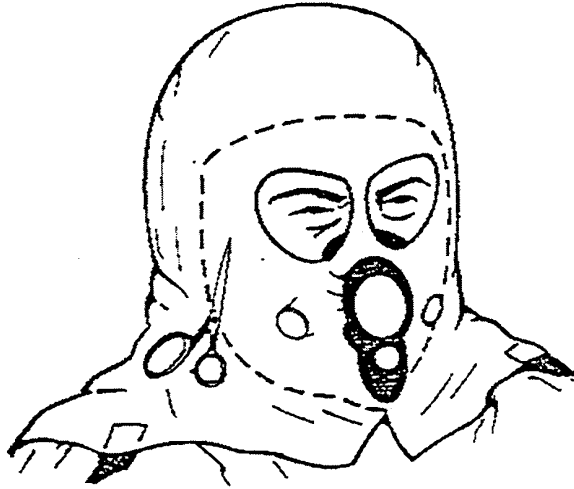
Figure 3-1. Cutting off the hood.
